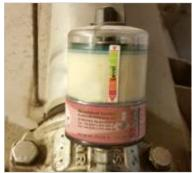
Refilling of the dispenser does not have to wait until the lubricant is completely empty; the dispenser can also be refilled seamlessly during normal operation.
