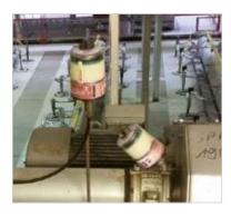
The running time per filling is adjusted directly on the device. The remaining filling cycles are shown by LEDs.
